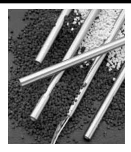
The Watlow EB cartridge heater is a proven performer like the metric FIREROD®. That's because the same quality materials go into its construction; MgO insulation, nickel-chromium resistance wire, silicone-fiberglass insulated lead wires. The only difference is that the EB cartridge is packaged in a more economical design. Instead of having the high watt density capabilities of a metric FIREROD, it's made for medium watt density applications.
