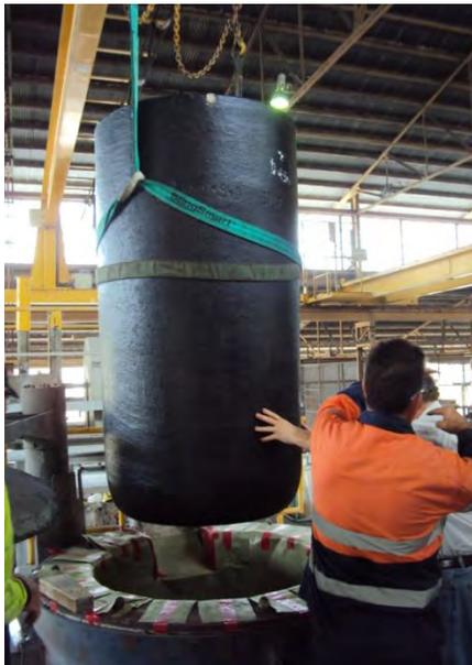
Fig. 3. A cylindrical crucible is installed in an induction furnace.
