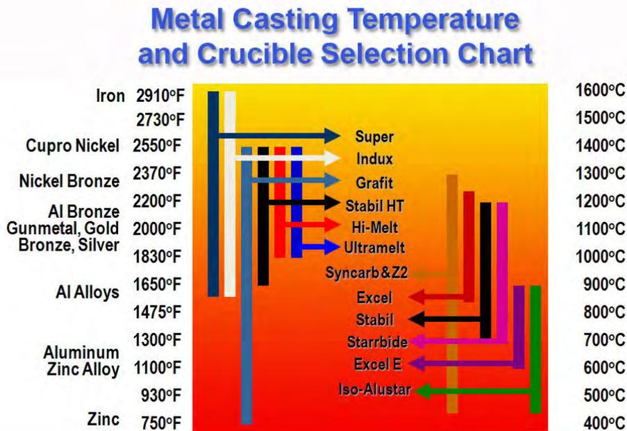
Fig. 4. A crucible must first support the range of metal temperatures it will encounter. But by offering products with overlapping temperature ranges, a crucible manufacturer is also able to provide a choice of crucibles with varying performance characteristics.
