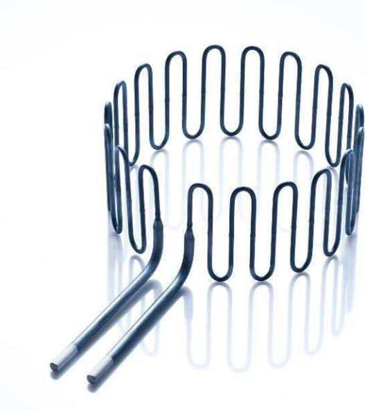
heating elements have a high purity glassy silica layer and this layer works as an oxidation protection layer with very low oxidation permeability. Therefore the heating elements show less deformation, an excellent low temperature oxidation (“pest”) resistance and long life use.
